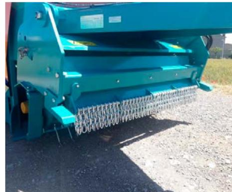
Before cleaning up the beach, the frontal pick up can be adjusted in three different positions.
